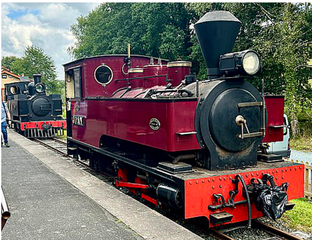
ASF no. 7 'JOAN' in her later guise as no. 14 'JOAN' on the Welshpool & Llanfair Light Railway in Wales. Apart from a tidying up of the front buffer-beam, the most obvious change is the removal of the two reciprocating pumps in front of the RH tank and above the rear of the LH tank.
