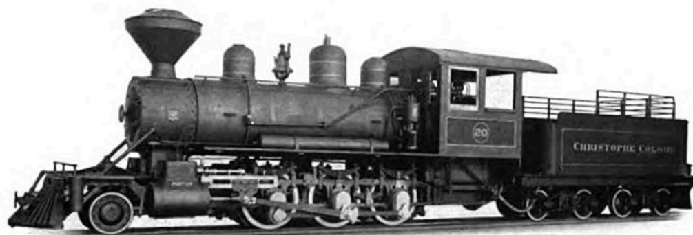
15" x 20" cylinders, class C-2-T, 30-inch gauge, engine 76,000 pounds weight and tender 47,000 pounds; air brake, wood fuel, outside frames and cranks. Exported to Haiti.
