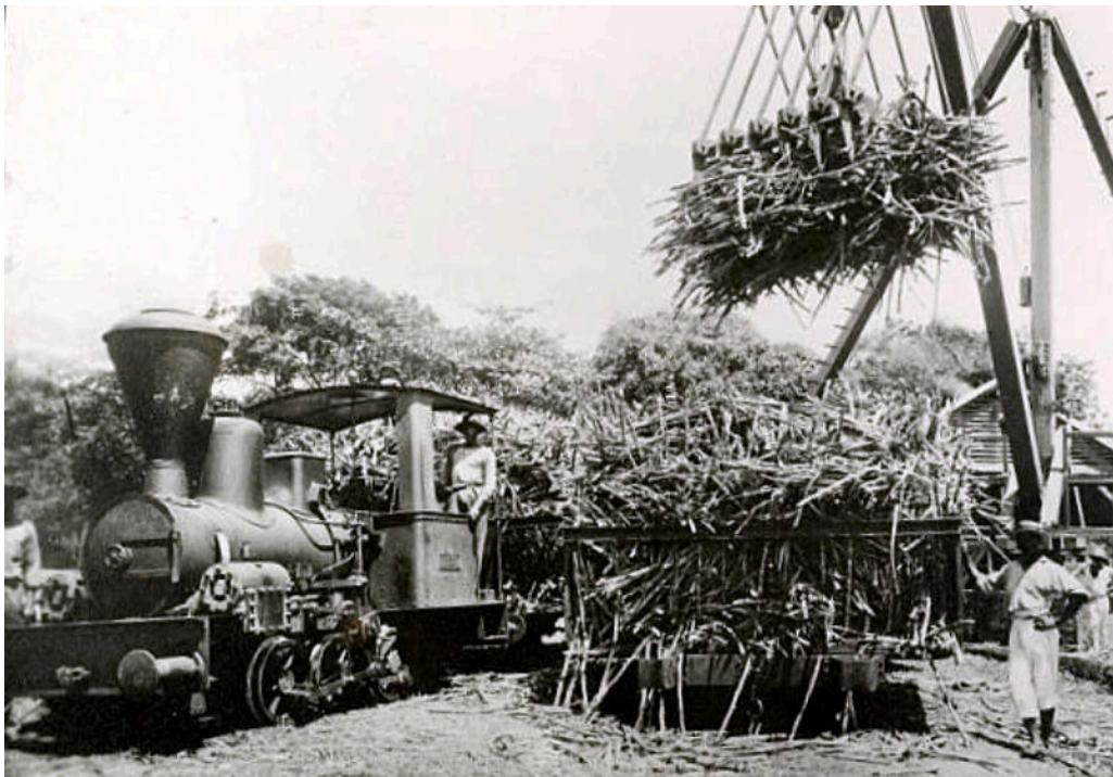
A Corpet-built 0-6-0T loco with Brown valve gear in use at Usine Ste. Marie.
