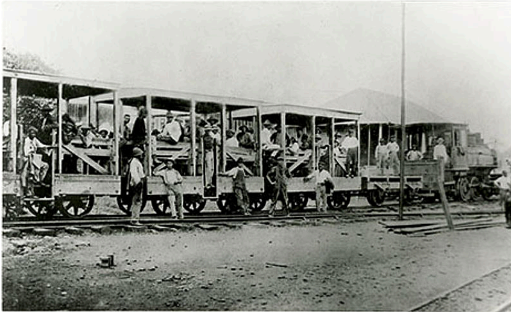
An American 0-6-0ST, probably from the latter part of the 19 th century, on a train of crude four-wheeled workers' carriages. This too is from the National Library of Jamaica Digital Collections, but might otherwise have been suspected to be in Panama where such locos and stock were common during the early days of work on the French canal project.
