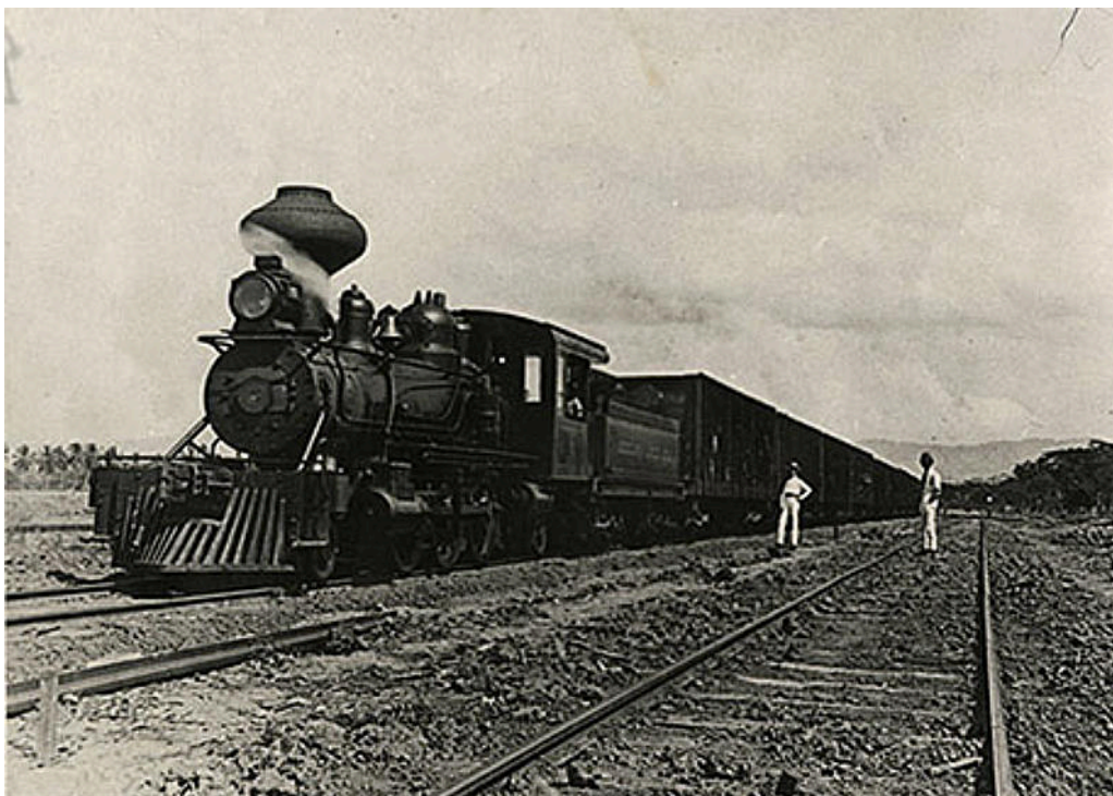
At a guess this is the Baldwin 2-6-2 listed above. The photo is from the National Library of Jamaica Digital Collections and was captioned as having been taken at Bernard Lodge which is just west of Kingston. It appears to be a 2-6-2, has a Rushton stack, and the name on the tender tank could plausibly be indeed 'KEELING-LINDO LTD.'
