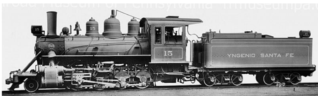
High res image available from the RR Museum of Pennsylvania: BLW neg no. 08910. Note the straight stack, though the spec. page had required a Rushton stack.
