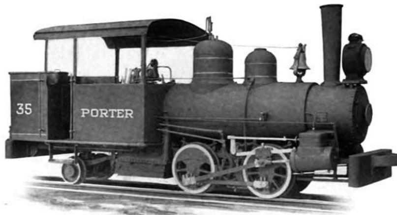
Illustration No. 35, from photograph of 8 x 14 cylinders, coal-burning locomotive, 30 inches gauge of track, for banana plantation in Jamaica.
