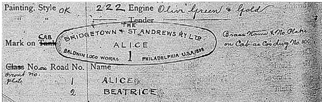
A portion of the Baldwin spec. page showing the combined name and number plates in standard Calthrop style. Annotations suggest that a detailed drawing of these had been supplied to Baldwin.
