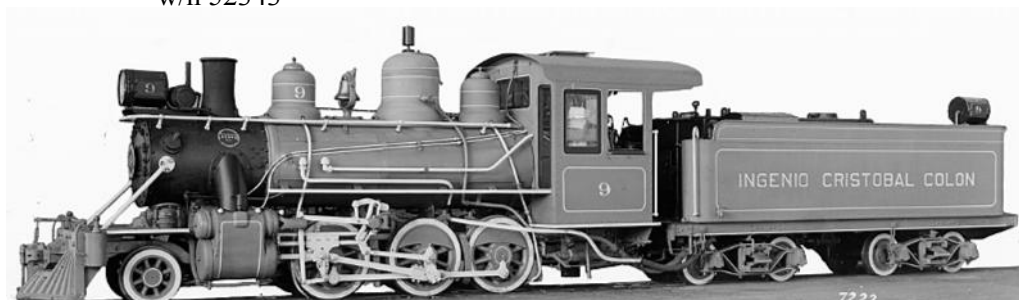
Ingenio Cristóbal Colón no. 9. High res image available from the RR Museum of Pennsylvania: BLW neg no. 07222-1. Note the extremely short chimney, which makes one wonder whether fitting of the Rushton stack visible in the photo below had been planned from the very start of the engine's life.
