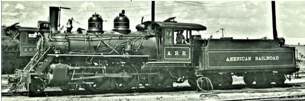
No. 72 in service, with the sand-dome having been moved back away from the chimney. Additionally a turbo-generator has been fitted, with an electric headlight, and the tender has been replaced by one with a less than full length collar. The chimney is now a stove-pipe. This is another Jack Delano pic from 1946, from the DeGolyer online collection.
