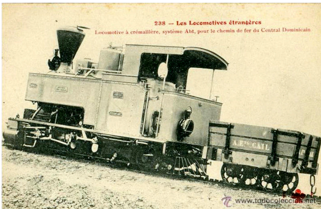
A well-known postcard of one of the FCD's Cail rack and adhesion tank locos, presumably based on a builders' photo taken before it left the Cail factory.
