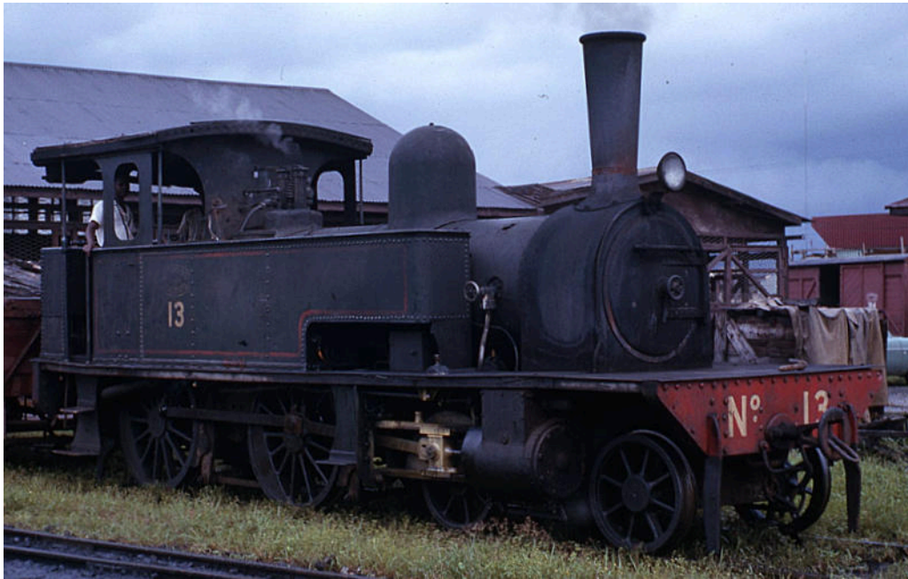
No. 13 during the 1960s, but still using link and pin couplers.
