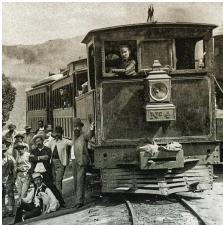
Loco no. 4 showing off its headlight, cow-catcher, and the Heberlein brake cable runners on the cab roof.
