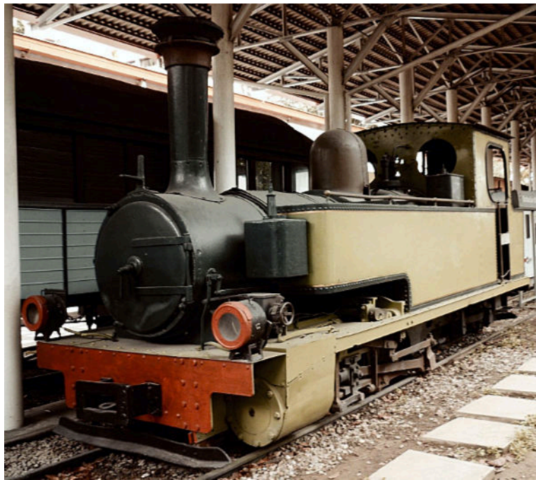
This is supposedly Hunslet 0-6-4T no. 8 , now in the Caracas Transport Museum, and very obviously built to a standard Avonside design but with an extended rear end and a trailing 4-wheeled bogie instead of a 2-wheeled truck. These photos are from http://www.forotrenes.com/foro/viewtopic.php?t=83296
