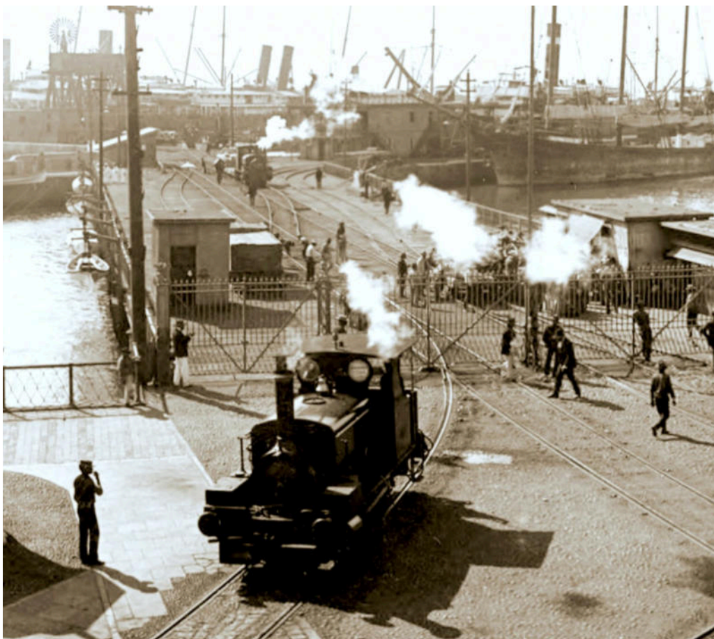
Two 0-4-OSTs at the entrance to Callao port. The nearer one has a saddle tank commencing behind the chimney, and the cab spectacle plate does not extend to the sides of the cab.
