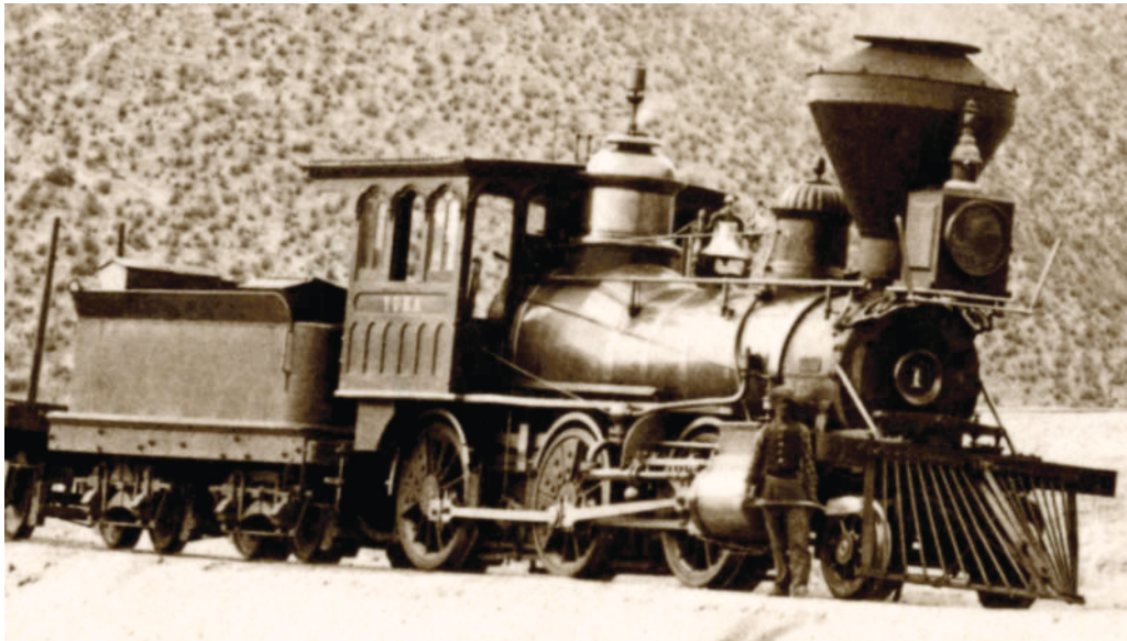
FCAyP Danforth Cooke mogul no. 1 'YURA' in a photo by Herr Alphons Stübel. Distinguishing features of these Danforth engines, when compared to the Rogers 1872 moguls, are the smokebox number-plates, the bolted-on multi-part wheel balance weights, the suspension cross-compensating beam in front of the smokebox, and the larger diameter of the steam dome. Source [14].
