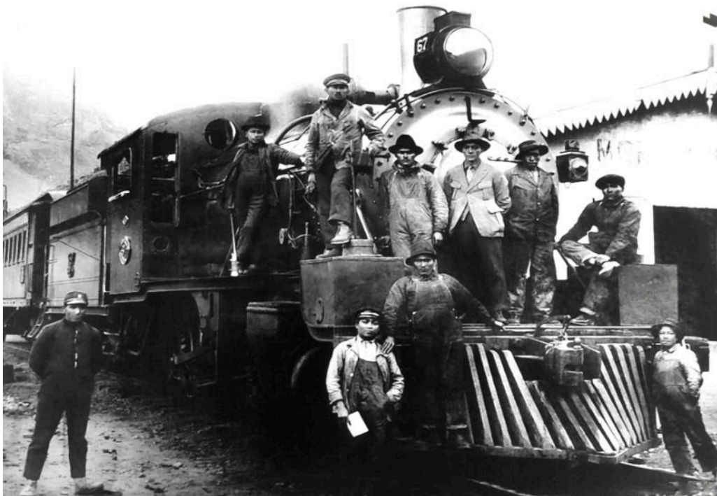
On the other hand, no. 67 was carrying buffer-beam-mounted sandboxes when seen at the head of a short passenger train at Morococha in 1936.
