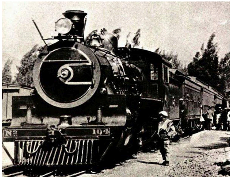
This loco numbered 104 would appear to be one of the ALCo 2-8-2s after undergoing the Anglicisation treatment seen earlier.
