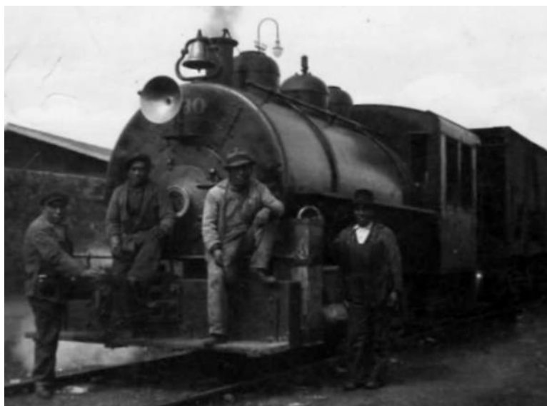
No. 30 . Note the full length saddle tank, which contrasts with the shorter tank on the later VIW-built 0-4-0STs.
