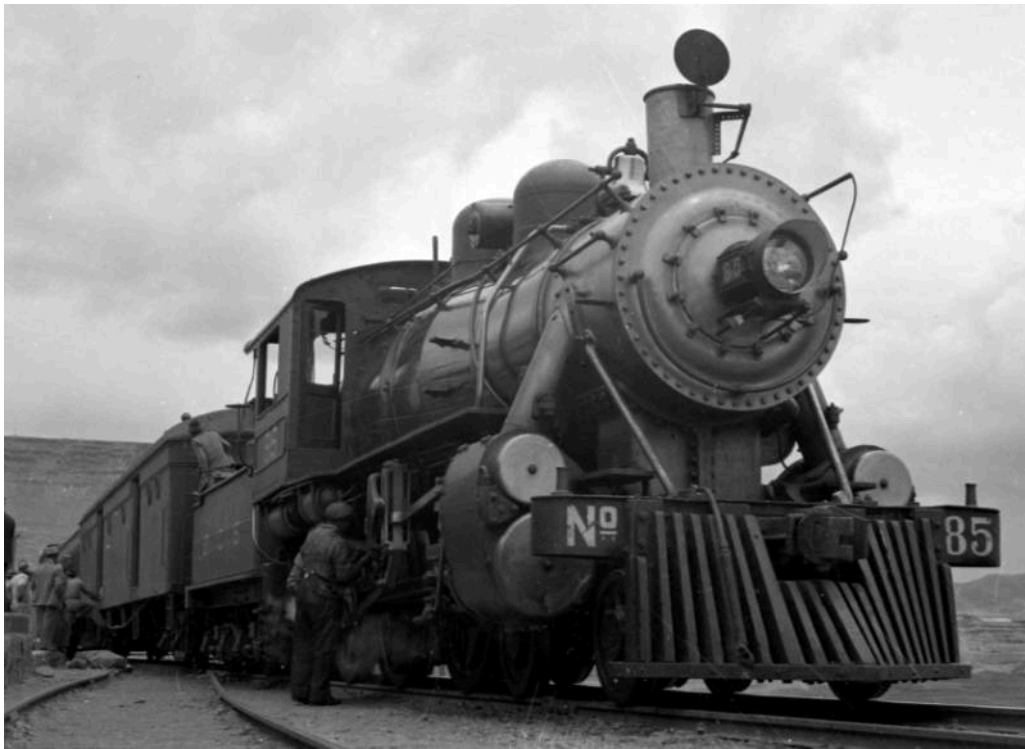
No. 85 even later in its career when rebuilt with new piston valve cylinders.
