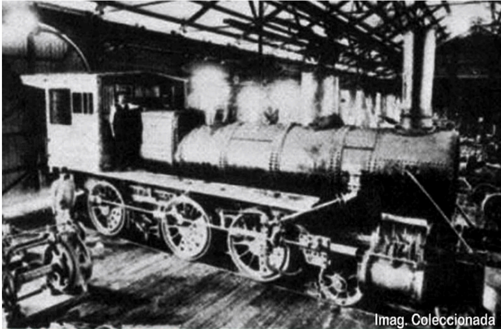
An unidentified 4-6-0 in the Arequipá workshops. Note the prominent belpaire firebox, the bolt-on balance weights on the driving wheels, and the apparent cross-head driven pump feeding straight to the clack. From Sr. Abrill Talevera's Amigos a los que les gusta Ferrocarriles y Tranvías Peruanos page on Facebook.
