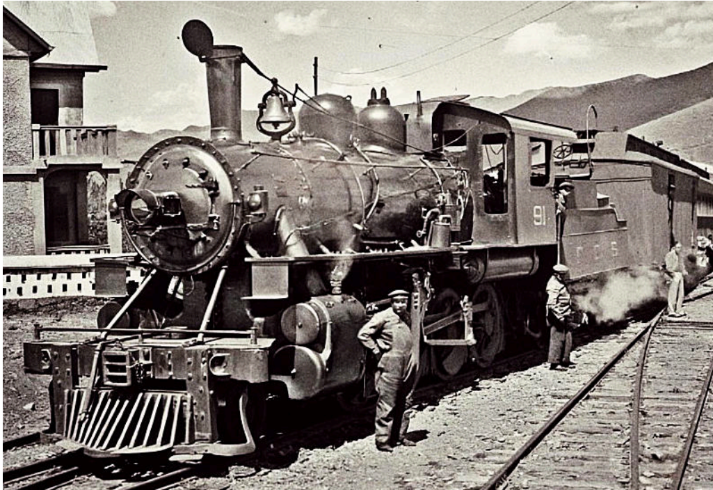
No. 91 at Wanchaq station in Cuzco in 1941. The loco still has its original link-and-pin coupler socket, and an ALCo style tender, but has been fitted with new piston valve cylinders and is missing the forward-mounted air reservoir seen in other photos.
