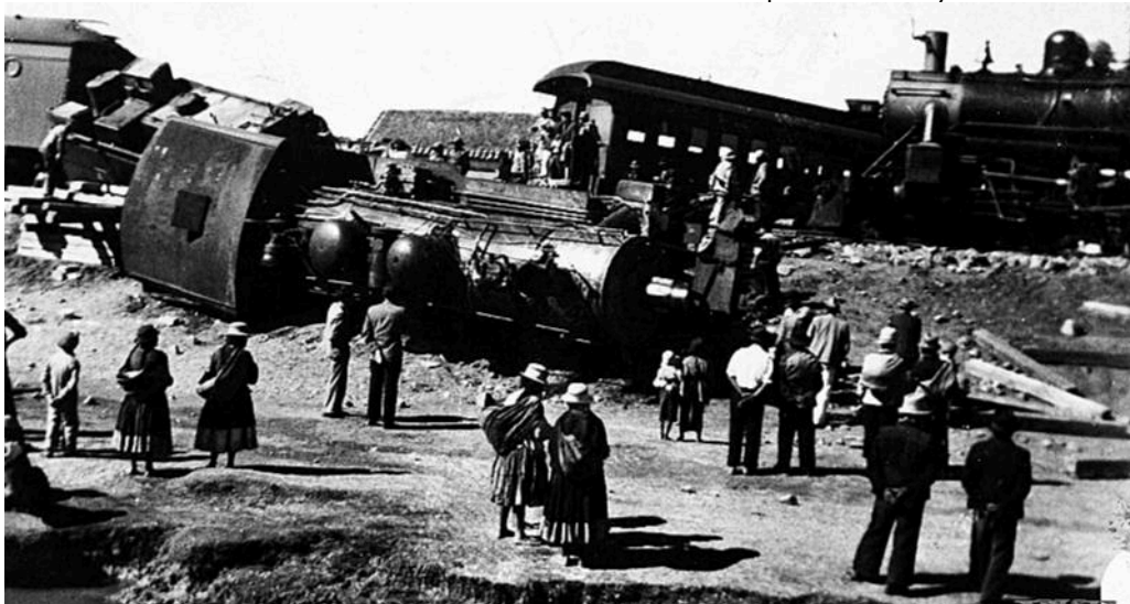
On 24th April 1946 there was a collision near Juliaca, seemingly between two passenger trains though this has not been confirmed. At least one of the two locomotives was an ALCo 4-6-0, and that is shown above and below lying on its side. The other engine in the picture above is also a 4-6-0 but it is not known if that had been involved in the collision or was a rescue loco.
