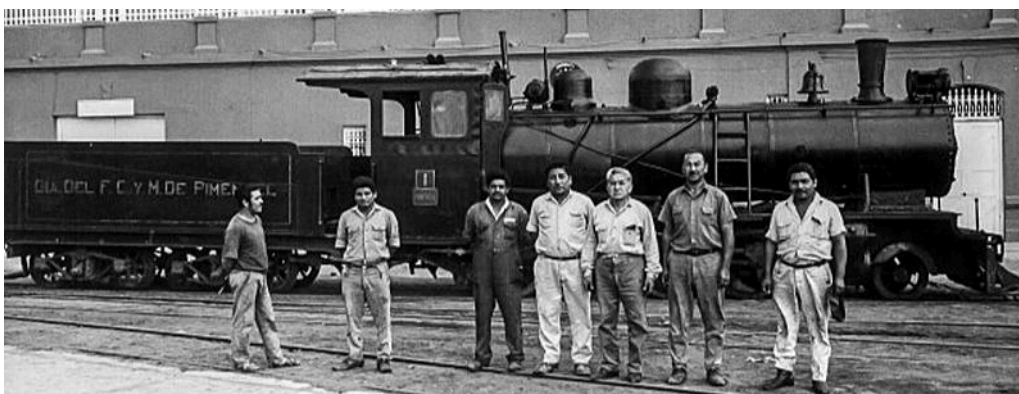
This image above shows the loco now with a straight chimney, with a rear sand-dome probably from a small US-built engine, but having lost the original front sand-dome. A ladder had also been fitted, probably for easy access to that front sand-dome.
