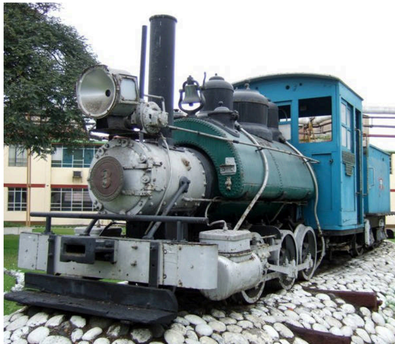
Note that no. 3 in its final plinthed state still retains the relatively tall steam dome that it was built with, in contrast to no. 2 .
