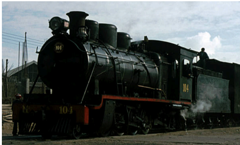
2-8-2 no. 104 leaves Huancayo in April 1975. Note the additional sand-dome when compared with no. 109 on the following page.
