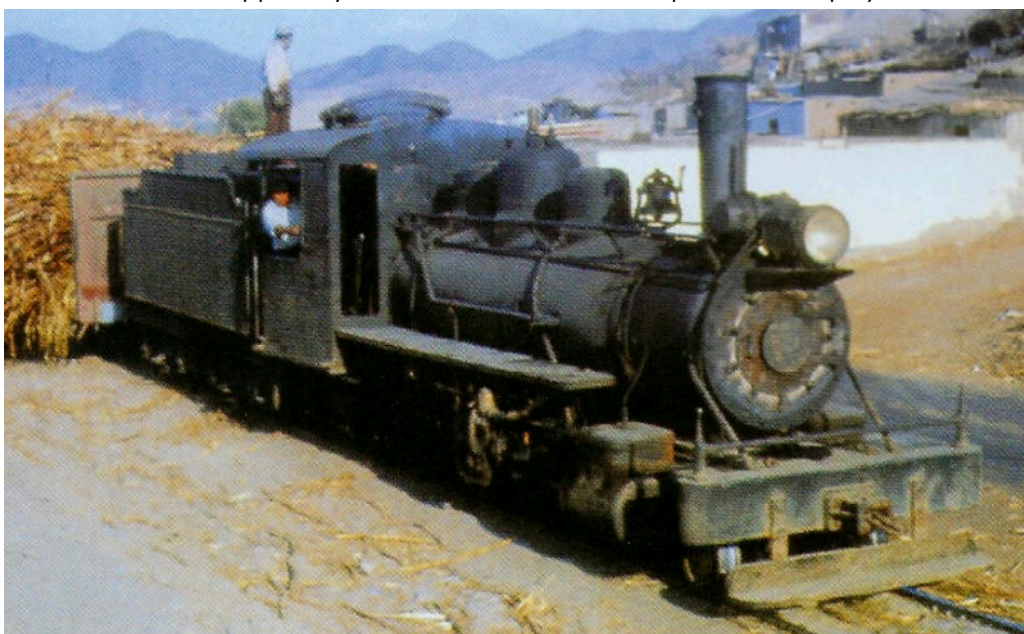
No. 6 on a cane train later in its life, and with a straight stack after conversion to oil firing. Photo by Thomas Walsh.
