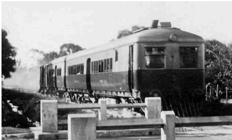
The two previous images showed Sentinel cars running with the power bogie trailing, but this photo has the power bogie at the front. It can be seen that there are no windows alongside the boiler, and the chimney and other roof features are also apparent. Behind the whole power car there would appear to be a trailer car and then a van.
