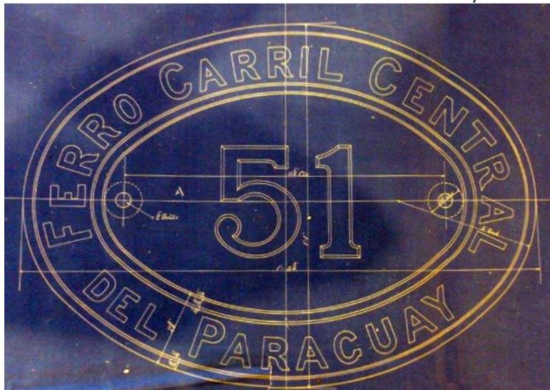
A blueprint drawing for the numberplates for this batch of engines, and an actual plate from no. 59. Note how the number spacing differs from the drawing.
