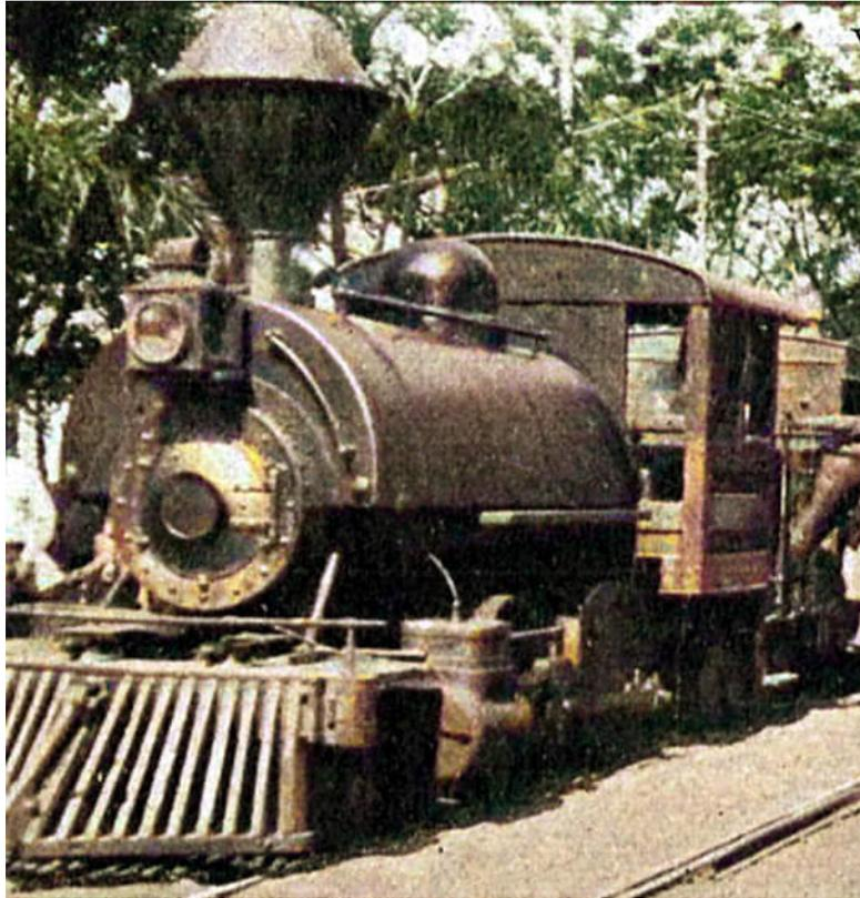
This tinted image shows a slightly different type of locomotive, with a dome. The saddle tank also extends to the very front of the smokebox, unlike in the previous photos. The tank has a wider profile too.
