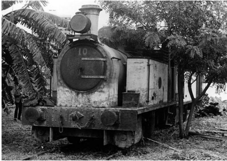
Disused 0-6-0Ts nos. **10** (above) and **11** (below) at ?? in ?. Note the gap in the rear bunker of no. **11**, with a chute to enable the transfer of wood fuel from a wagon or tender attached behind. Photo kindly provided by Richard Pelham.
