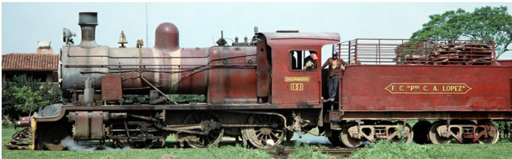
The most obvious distinguishing feature of these YECO engines was the wrapover cab roof. note that this engine has a conventional dome with sandboxes on the running boards rather than the combined elongated dome originally fitted.
