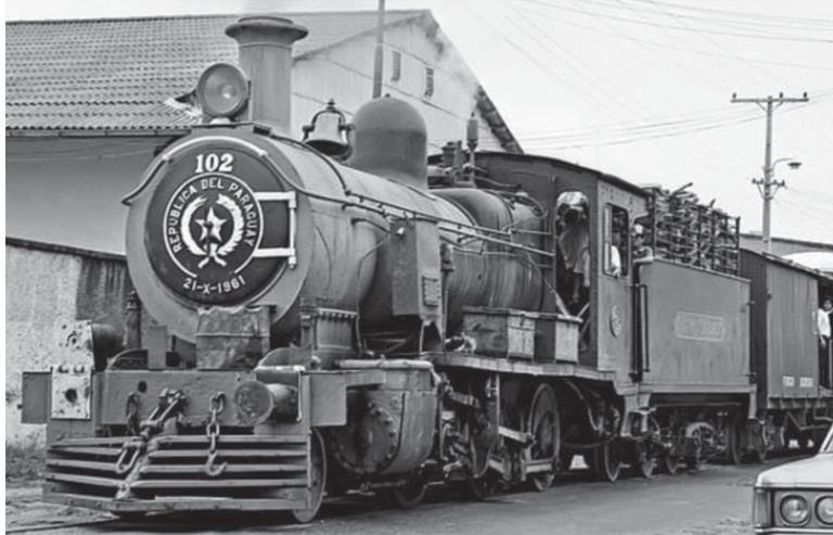
This street running view of no. **102** interestingly shows one of the front buffers folded up and the other down. The boiler side sandbox is also clearly visible.
