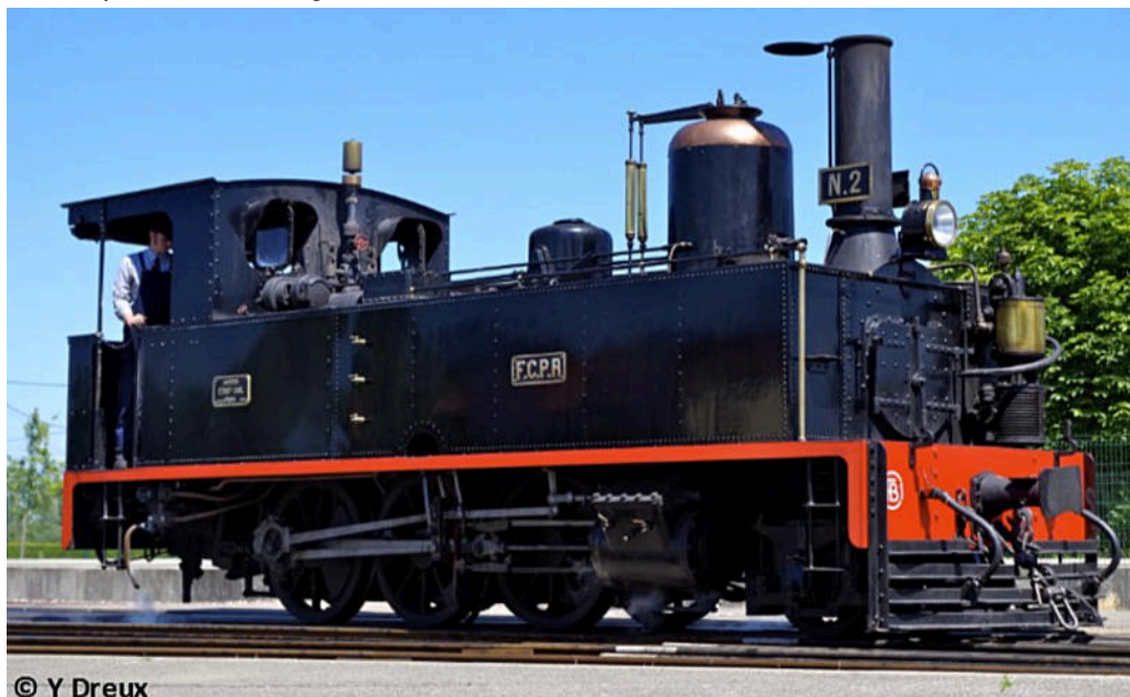
No. 2 as it is nowadays, back in France and running at the Chemin de Fer de la Baie de Somme . An air-pump and turbo-generator have been added, when compared with the image above.
