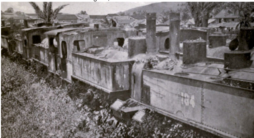
Several lines of locos are visible here, with Franco-Belge 0-6-0T type 88s or the equivalent in the nearest row, including no. 184 nearest to the camera.
