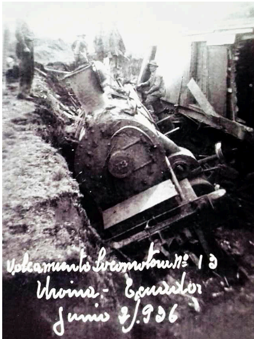
And another mogul derailed; this time no. 13 in June 1926, and showing that by then it had received 'bolt-on' piston valve chests.
