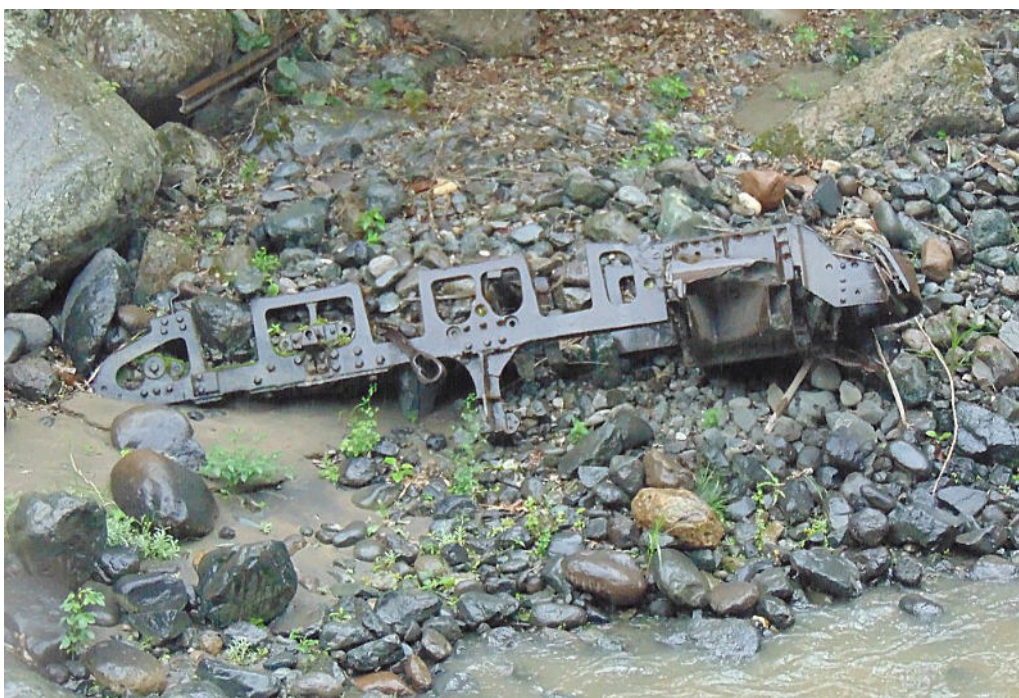
A bogie frame from a Garratt still lies in the Chan-Chan river 500m south of Estacion Ochoa. This may have been from no. 102 after its accident at Km. 105, and makes one wonder whether the engine ever worked again.
