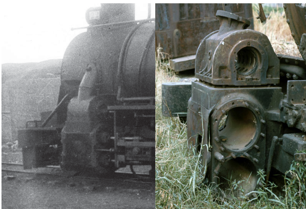
The cylinder blocks from the Vaucrain four-cylindered 2-8-0s were modified by having 'bolt-on' piston valve chests affixed in place of the original slide valves to improve their efficiency. The left hand image shows no. 22 in that modified state in 1936, whilst the right hand photo shows a derelict loco's modified cylinders and valve chest in the yard at Duran in 1975.
