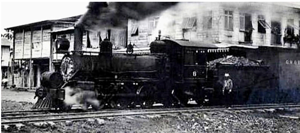
Two views of 4-6-0 no. 6 , identifiable by its dome over the firebox, a feature which distinguishes it from all the later G&Q locomotives.
