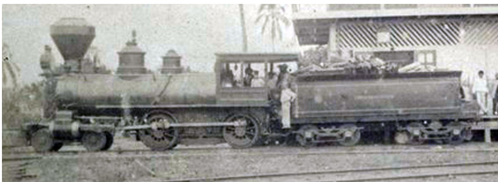
This photo at Yaguachi station shows a 4-4-0 but one very different from the machines illustrated earlier. This is probably loco no. 5 . Note the steam dome ahead of the sand dome, a very unusual feature and one not seen in any other photo in this section. The Baldwin spec. sheet for no. 5 does specify a straight boiler and the dome to be in the forward position.
