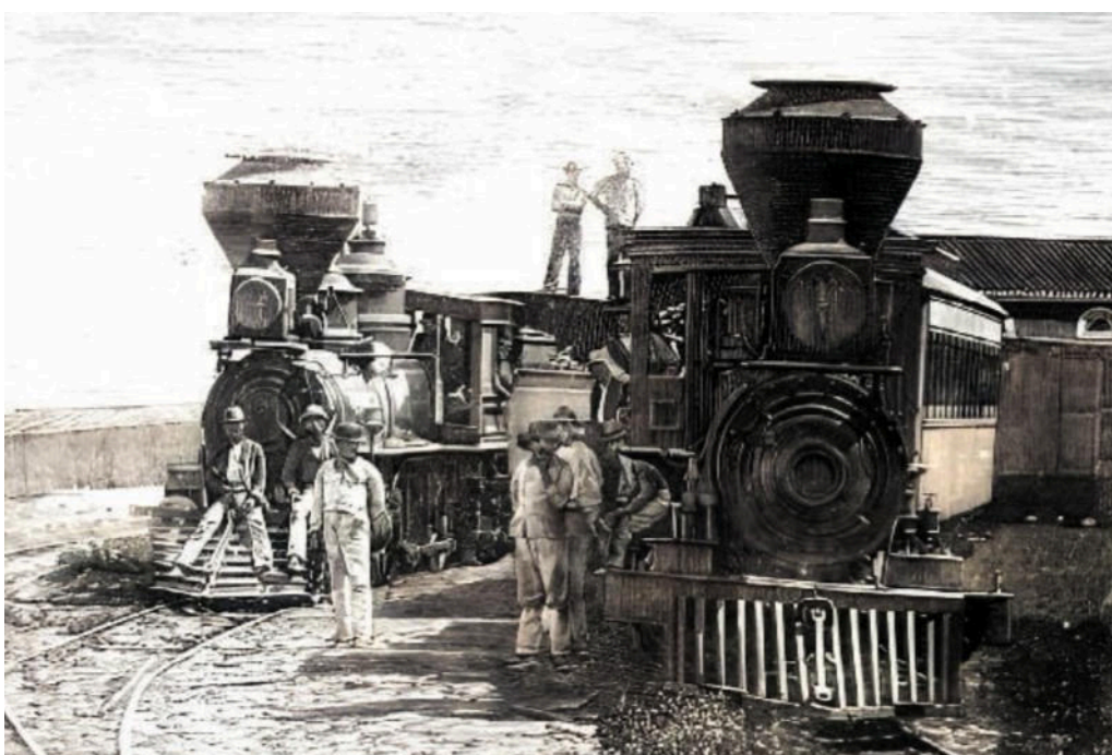
The right hand engine seen here might well be that in the previous picture, for the proportions, height of running board, etc. are similar. The left hand loco, however, is clearly different, with a running board well below the boiler centre line and boiler and dome mounted much higher.
