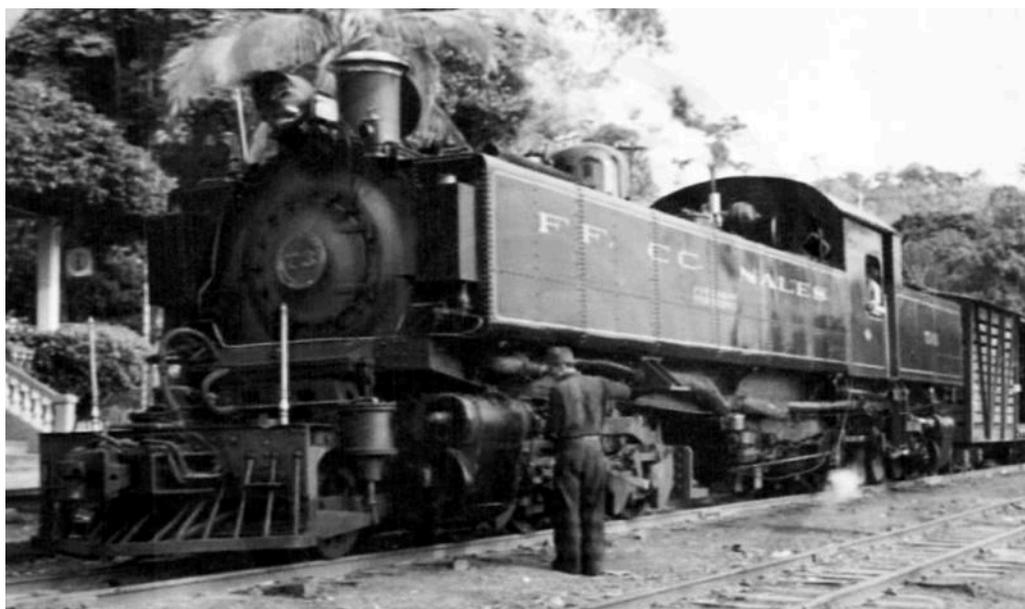
Careful examination of this photo showing one of the 2-8-8-2T Kitson-Meyers on a train reveals that the cab roof has been raised considerably, though the side window remains in its original position. The tank side inscription appears to read 'FF. CC. NALES' with perhaps 'CENTRALES' beneath. The smokebox number clearly finishes with a '3' and is therefore probably **173**.
