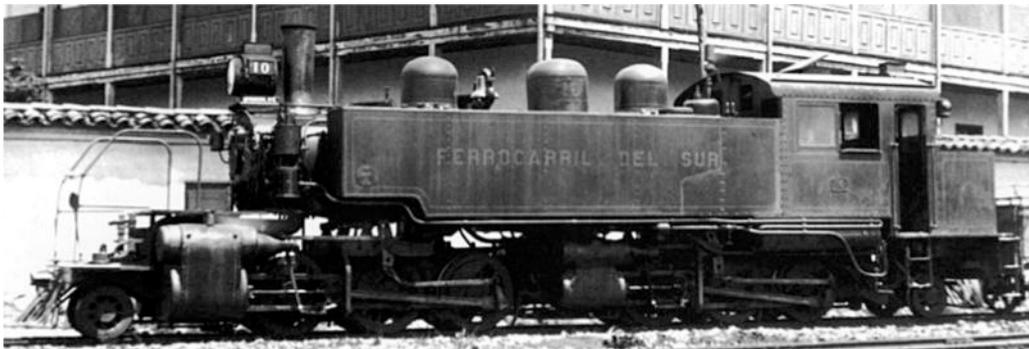
P. C. Dewhurst's photo from 1925 shows no. **10** missing its turbo-generator but having gained front handrails. [8]
