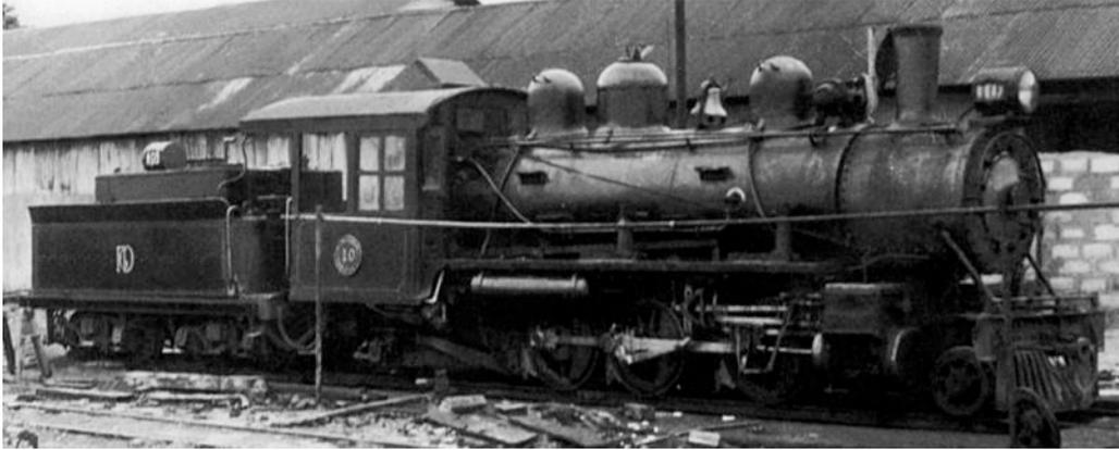
The original no. **14**, as renumbered **10**, as seen at Mariquita workshops around 1958. [8] The oil tank, cabside number-plate, and turbo-generator and headlight are the main differences from the loco as built.
