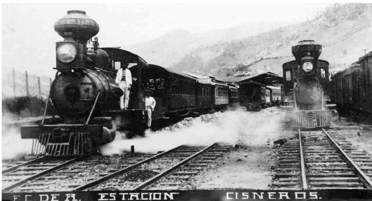
Two of the Baldwin 2-6-0s of the FC de Antioquia. On the right no. 14 carries a Radley & Hunter stack, whilst its unidentified sister on the left has a Rushton stack.
