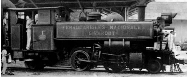
FC del Tolima 2-4-2ST no. 15 by Tubize after rebuilding with side tanks and now as FCN Girardot no. 1. [8]
