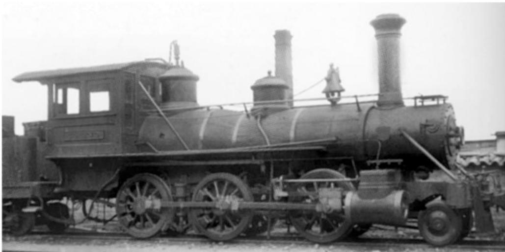
A P. C. Dewhurst photo of no. 6, sourced via [8]. Note the slightly different design of dome from the previous photo, the lack of a headlamp at this late stage in the loco's life, and the bracing rods to link running plate to cab.
