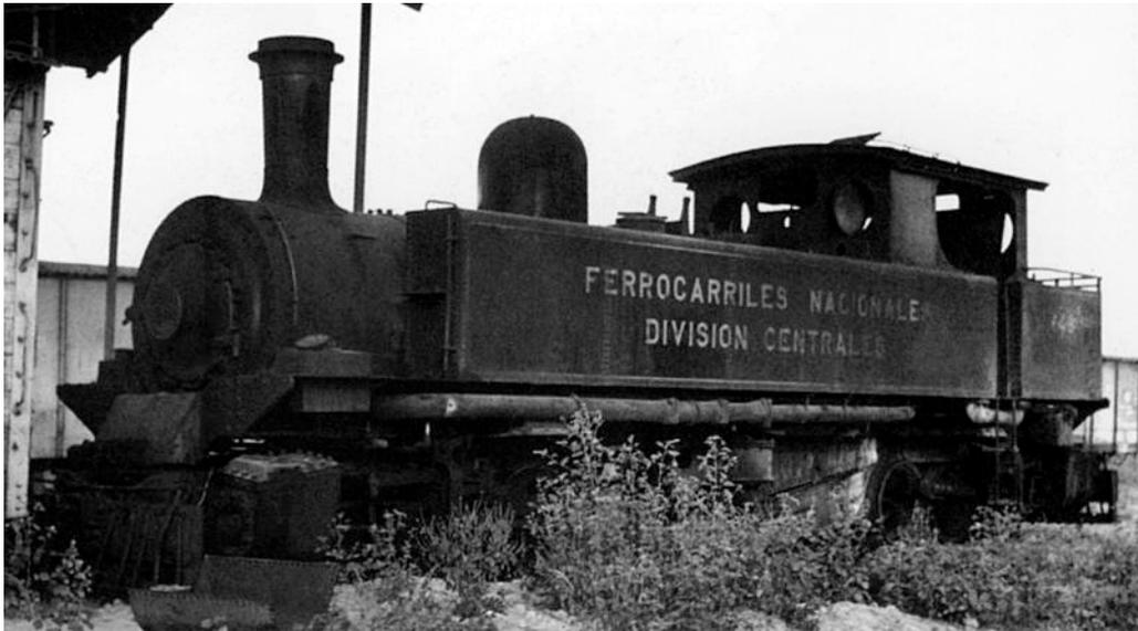
This is supposedly FCN-C no. **149**, ex FC de Girardot no. **21**, lying at Facativá in 1955. [8] Note that the front ends of the tanks are further back relative to the smokebox than when first built. This loco has a replacement front bogie, fitted cylinders forward.
