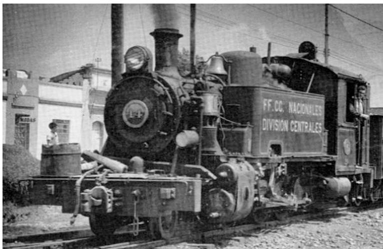
FCN-C 2-6-2T no 14 built by BMAG and originally owned by the *FC del Sur* and later by the *FCNyNE*. This photo was taken by Gordon Crowell and was published in Whitehouse and Allen's *Round the World on the Narrow Gauge* in 1966.
