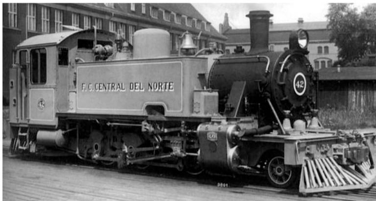
The first of the 2-6-2Ts for the *FC Central Norte Segundo*, no. 42, before delivery from *BMAG*. [8]
