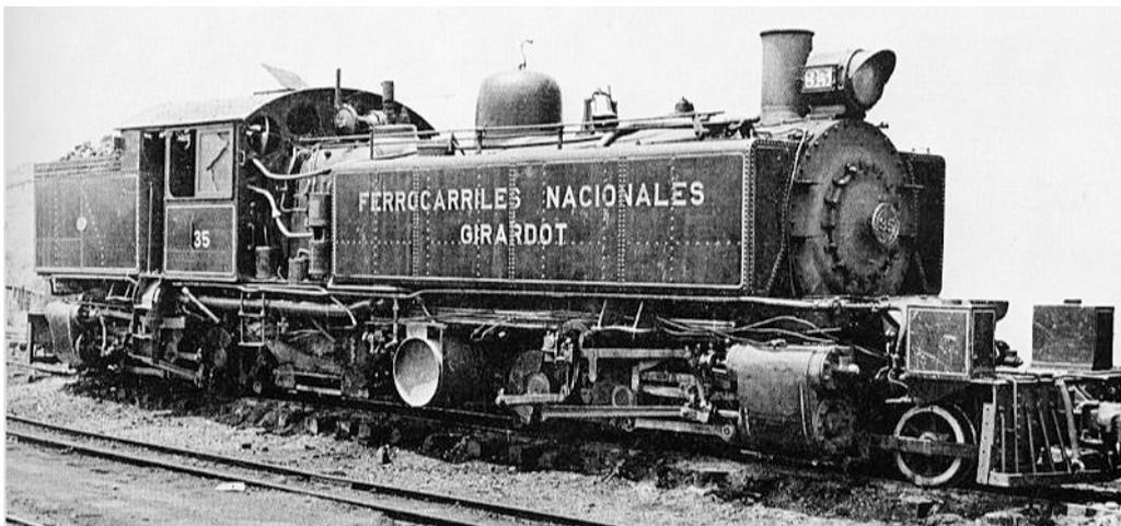
Whilst the basic design of this engine is as for those pictured above, there are clear differences. The cab has higher eaves and a larger side window owing to the railway's loading gauge having been enlarged, and sandboxes have been added above the front pony truck. Nevertheless it is one of the four 1927 locos, albeit with the running number **35** which no. **24** gained after the merger with the FC Tolima - Huila.
