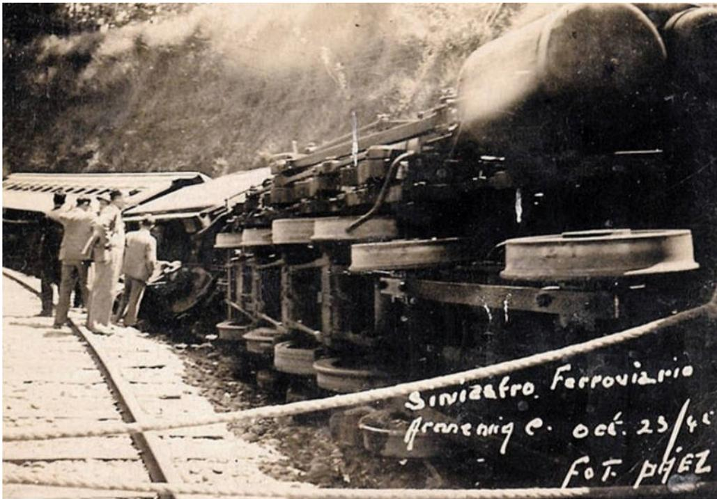
**2-8-2T d/w 37", cyls. 16½x20", built by BMAG in 1927 and 1928**
