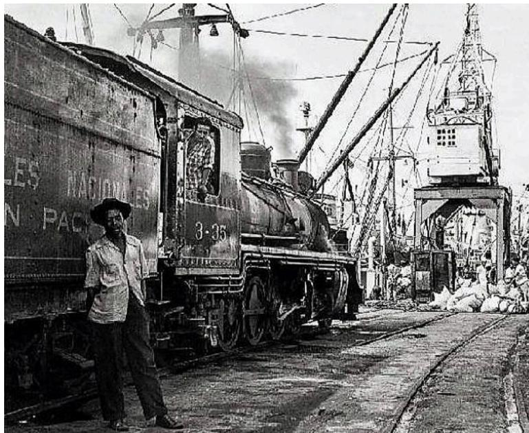
No. **6**, ex *FC de Caldas* no. **6**, an ALCo 2-8-2, as renumbered **3** and also displaying its adhesive weight of 35 tonnes.
