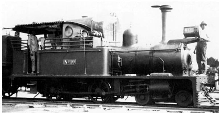
No. **19** as captured by PCD. [8] Note the longer smokebox than in the image of no. **16** above.
