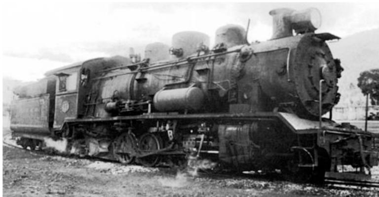
No. **02**, showing the air reverser above the running board ahead of the firebox. [8]
