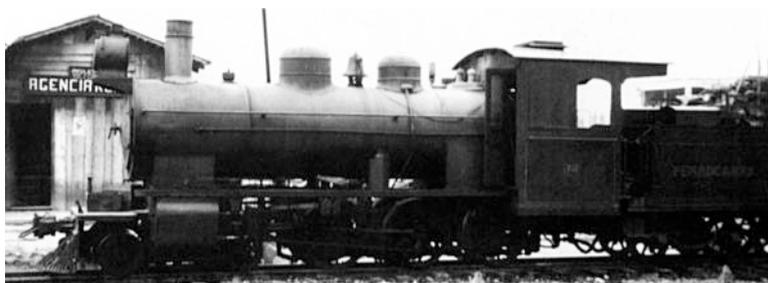
A later photo of no. **32**, with a chimney extension, a bell between the domes, and seemingly the foremost of the cabside windows blocked up.
