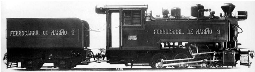
The final two also had small four-wheeled tenders, and thus were not fitted with the wood rails above the tanks. This one is no. **3**, as seen in a HanoMAG works picture. [8]
