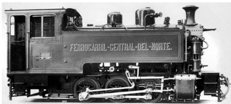
FC Central del Norte Segundo no. **33**, as seen in a HanoMAG works photo. [8] These were very similar to the locos supplied by HanoMAG to the *FC de Nariño*.
