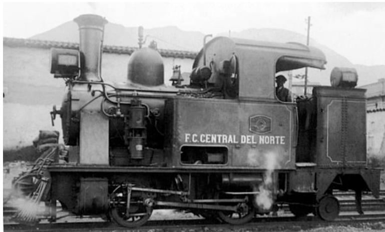
Like many other railway systems, the Colombians seem to have found steam railcars very limiting in that any necessary maintenance knocked out both loco and coach from use. Thus this one was rebuilt as a 2-2-2T. [8] Photo by P. C. Dewhurst.
