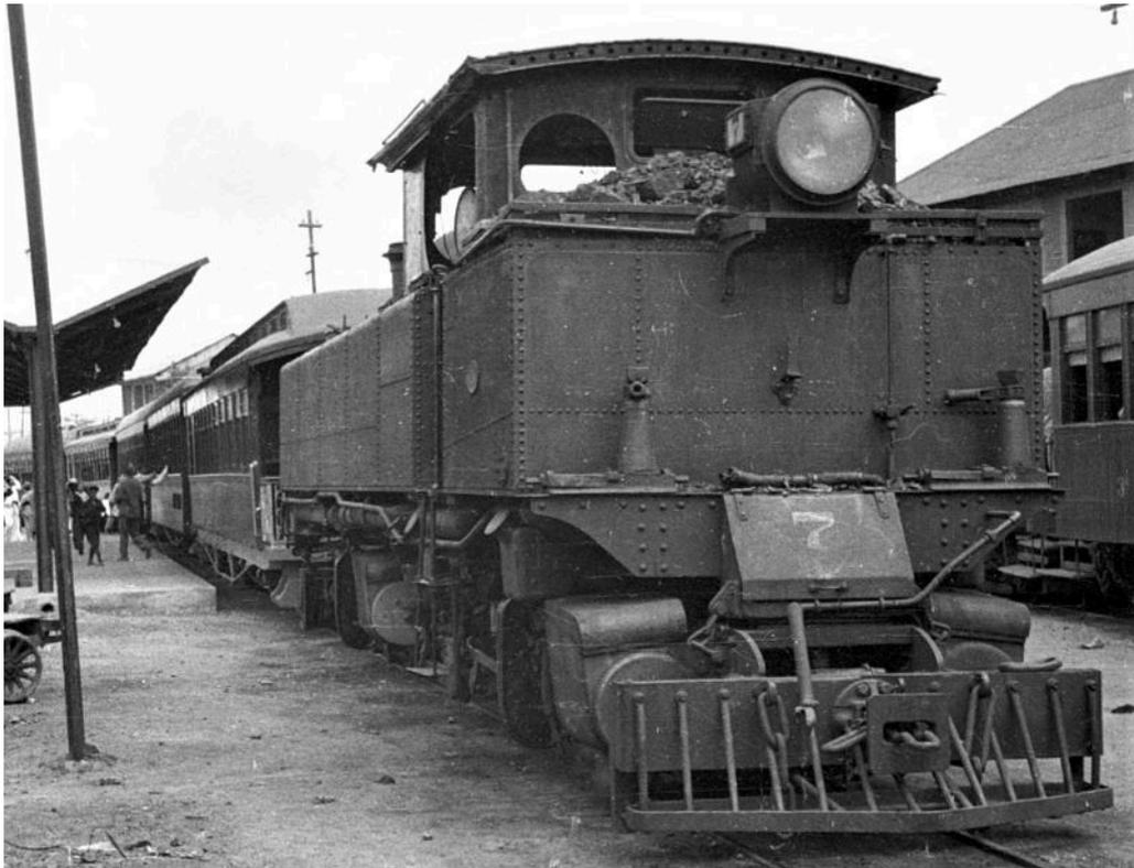
No **16**, as renumbered **7** and seen at the head of a passenger train at Girardot in 1933. However, it has lost its lifting eyes, and might therefore have experienced the usual swopping of parts.
