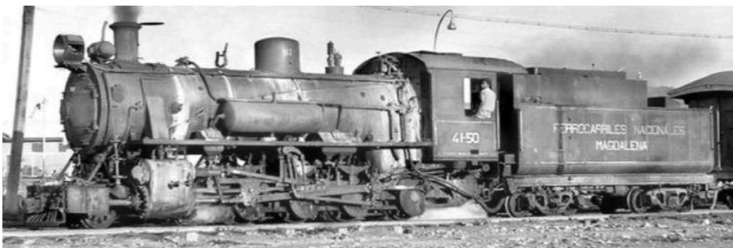
No. **41** in the FCN-M era seen bearing the double number **41-50** indicating an adhesive weight of 50 tonnes.
