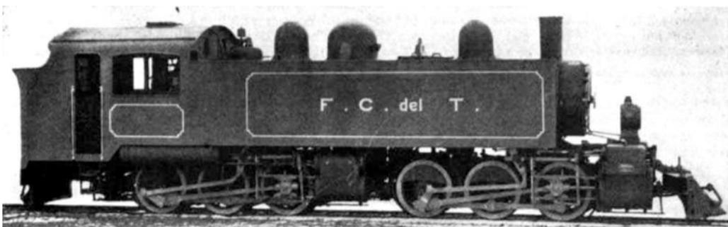
A photo from an ALCo publicity card. Whoever created the lining-out obviously was too familiar with the actual construction of the locomotive, for the whole point about the fairing between tank and cab was to give the impression that the tank continued back to the front of the cab.
