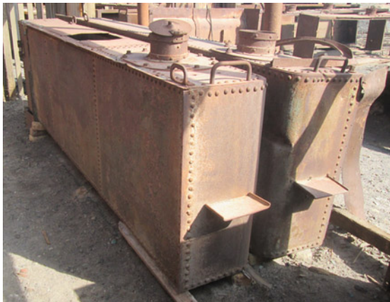
LH Tank 351cm length, 117cm height, 45cm thick,. RH tank Similar to group 16 but with a different filler, see group 16 for dimensions
