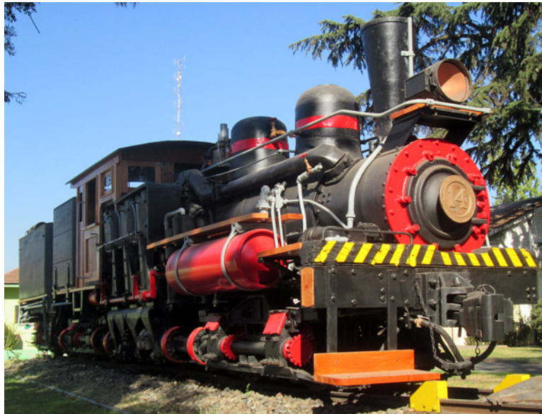
No. 14 as seen in April 2019, after repainting and the replacement of the woodwork including the cab, running boards, buffer beams and switchers' platforms. It can be seen that this loco is also superheated, as evidenced by the large diameter steam pipe leading back from the smokebox to the engine unit.
