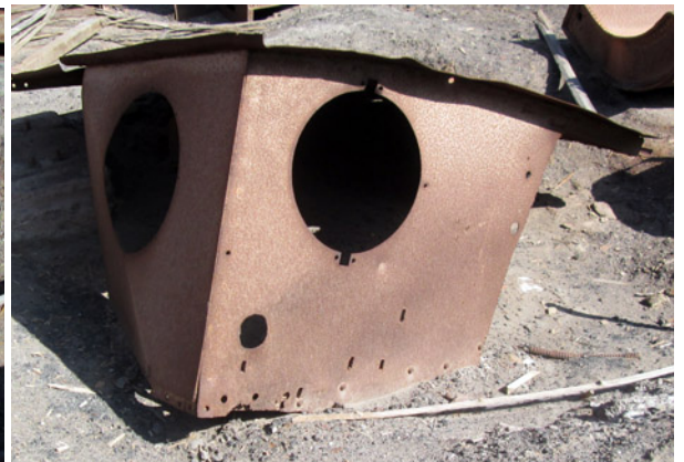
Cab 222cm length of roof, 102cm length of side panel, 89cm height to eaves, 47cm diameter of porthole. Safety valves came up though roof. Possibly by Manning Wardle? MW 0-6-2Ts 1764-5 supplied to Colorado Nitrate had side portholes like this one.
