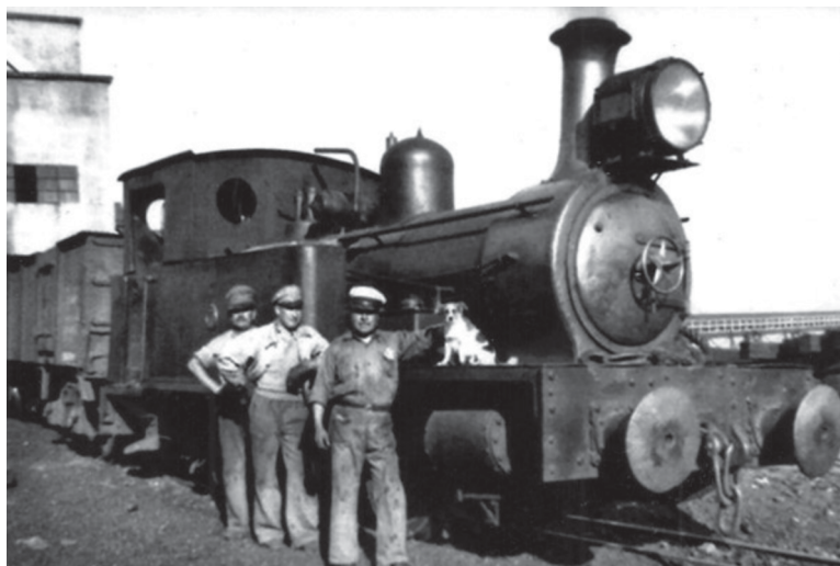
One of these three locos in use, seemingly with a slightly taller chimney than in the photo above. The engine is standing on mixed gauge track and the sheer size of the bogie coal wagon behind it suggests that it may have been a broad gauge vehicle belonging either to the EFE
