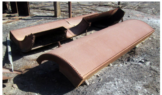
Saddle tank 320cm length, 128cm distance of dome c/l from one end, 98cm top to bottom. This might be from one of the FC de Agua Santa 2-4-2 STTs by Baldwin.
