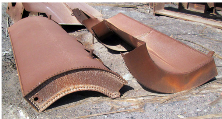
Saddle tank 320cm length, 128cm distance of dome c/l from one end, 98cm top to bottom. This might be from one of the FC de Agua Santa 2-4-2 STTs by Baldwin.
