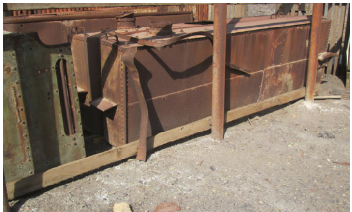
LH Tank 351cm length, 117cm height, 45cm thick,. RH tank Similar to group 16 but with a different filler, see group 16 for dimensions
