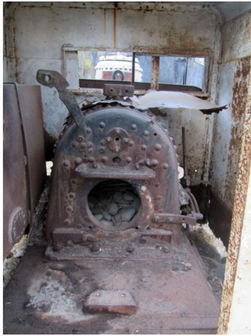
The cab of the surviving loco at Balneario Cachapool. The oil tank filling the left side demonstrates why there are no windows on that side.
