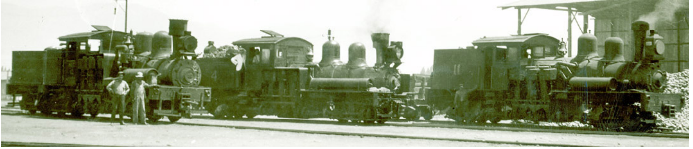
Three Shays together, including on the right no. 11 which can be seen to be more solidly built than no. 4 in the middle. No. 10 is on the left. All three engines retain the cast link and pin coupler blocks with which they were probably delivered.
