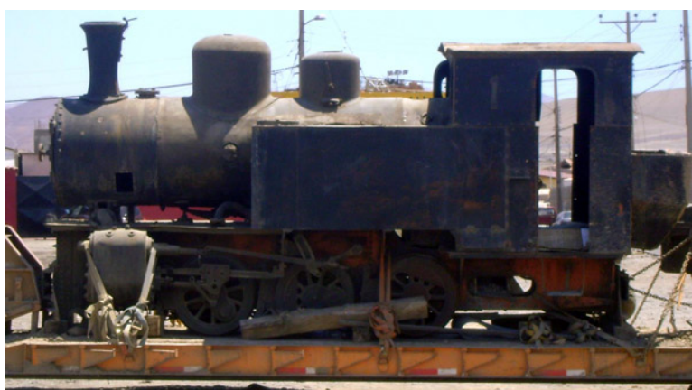
The Rheinmetall 0-6-0T on a low loader in Arica whilst on its way south around 2012. Close examination reveals a very clear number '1' on the upper cabside where a metal digit had been removed. Note also the added rear bunker cantilevered out from the cab.
