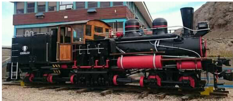
No. 5 as recently repainted and with new woodwork, at Alto Colón in 2019. The loco still carries its dual height couplers.
