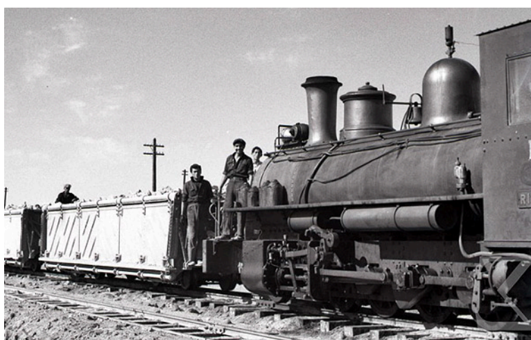
Hunslet 1480 no. 1 'RITA' , seen on a train of caliche hoppers at oficina María Elena, supposedly in the 1950s. Note the added bell, and the turbo-generator in front of the chimney.
