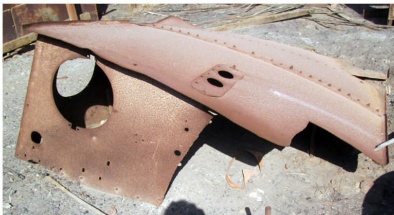
Cab 222cm length of roof, 102cm length of side panel, 89cm height to eaves, 47cm diameter of porthole. Safety valves came up though roof. Possibly by Manning Wardle? MW 0-6-2Ts 1764-5 supplied to Colorado Nitrate had side portholes like this one.
