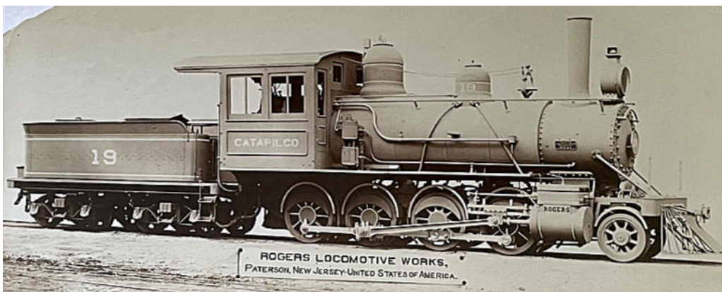
A Rogers publicity card photo, again showing no. 19 'CATAPILCO' with the straight-topped cab windows. This suggests that it was built like this. However, note the different chimney to that shown in the previous image.
