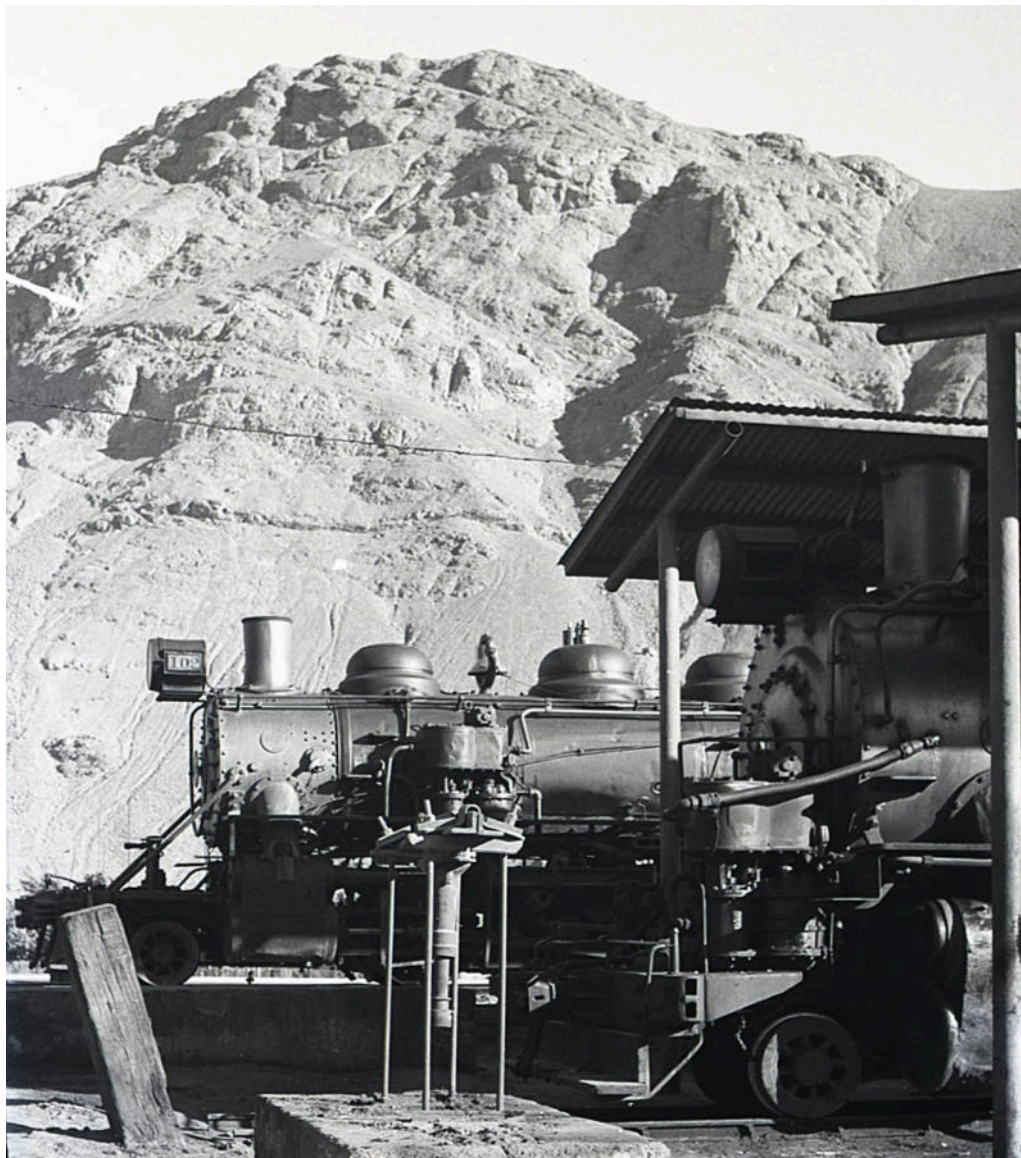
Two locos on shed at Llanta, in the foreground is one of the 50-53 series 2-8-2s, which had their air-pumps mounted right forward, whilst further back is no. 102 , one of the three 2-8-0s which carried their pumps much further back alongside the boiler.
