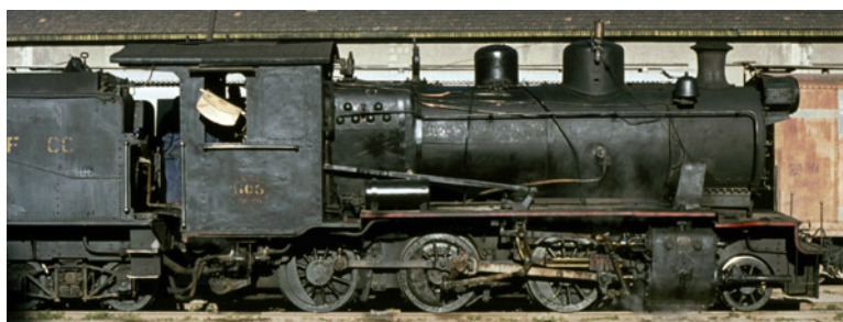
Ex-FCALP Henschel 2-6-0 no. 15, running as ENFE no. 505, shunting at La Paz in 1975. Note the slightly raised running plate, and the steam/air-operated bell on the smokebox.
