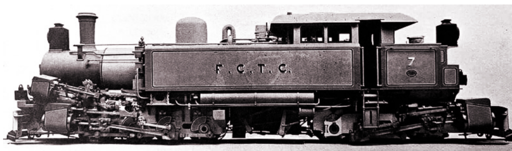
No. 7 as built, showing the additional rack cylinders alongside the smokebox, and the small bunker.
