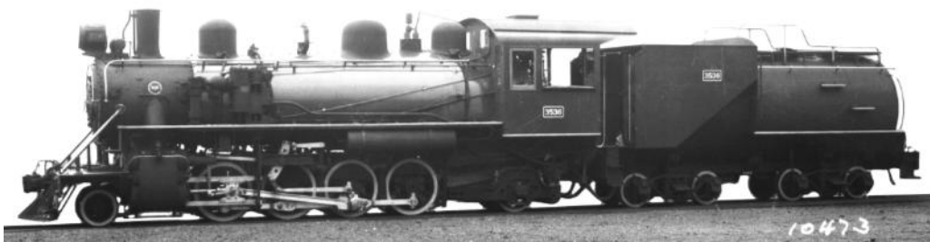
No. 3536 , with a B, B-2, BL, or BL-2 Worthington feed water heater mounted on the fireman's side, and probably with the air pump relocated to the driver's side.
