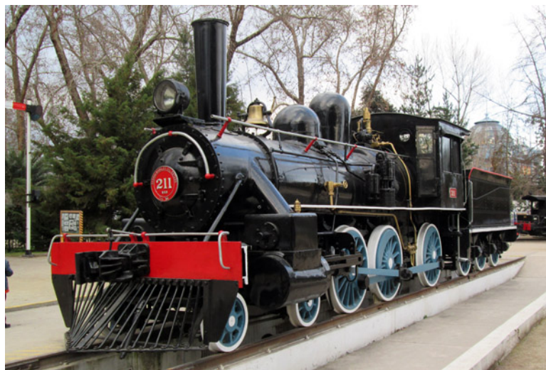
MCC's own photo, taken at Quinta Normal museum. Note the bolt-on piston valve chests, in place of the original slide valves. Note also that the dome is further forward than in the previous picture, implying that reboilerings were done with a modified boiler design.
