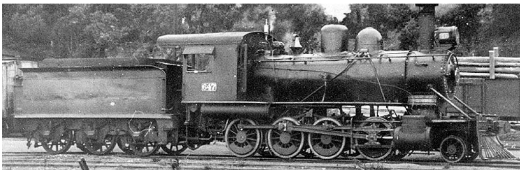
Tipo 69 no. 647 . The replacement boiler has been mounted higher than the original, probably because of a deeper firebox. The additional height of the smokebox above the saddle casting can be seen, also the shorter smokebox and round-topped firebox.
