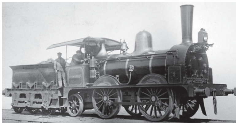
No. 2 ' VENCEDORA ' now with a flared stovepipe chimney and an air pump in front of the cab. The wheels are larger than those in the photo above (perhaps by 6") as evidenced by the greater distance of the footplate from the trailing wheel flange, the slightly deeper buffer beam, and the relative heights of the loco and tender running plates. The sandboxes are also larger than those seen above.
