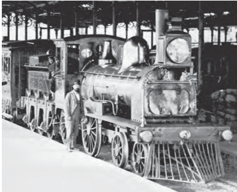
Number 4, rather later it would appear, with a rather more substantial cab and a boiler with dome much further forward.
