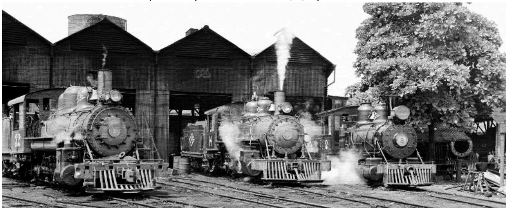
Probably again at Sonsonate, but this time with one of the ex-Hawaiian 2-8-0s on the left. Note the knuckle coupler fitted to those engines in contrast to the link-and-pin fittings which the older engines were equipped to the last.
