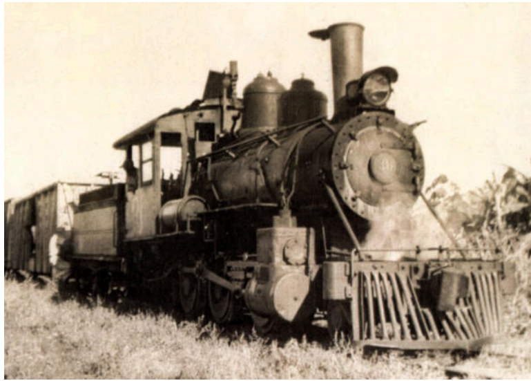
A 2-6-0 numbered 30 , but not yet positively identified as one of these. It has been retro-fitted with 'bolt-on' piston valve chests.
