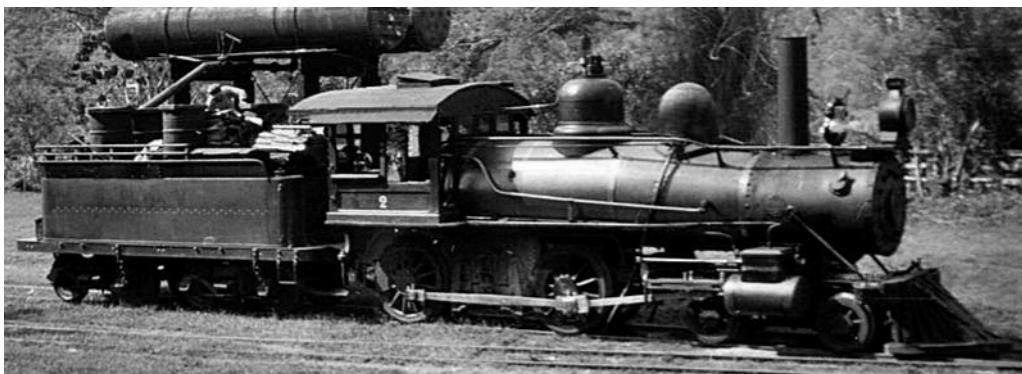
These next three photos again show no. 2 'COBAN' , but the engine has now been reboilered and now has a wider steam-dome with a conventional Baldwin wider mounting ring and mounted further forward than the original.
