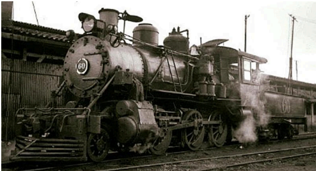
No. 60, as later retro-fitted with piston valve cylinder blocks.
