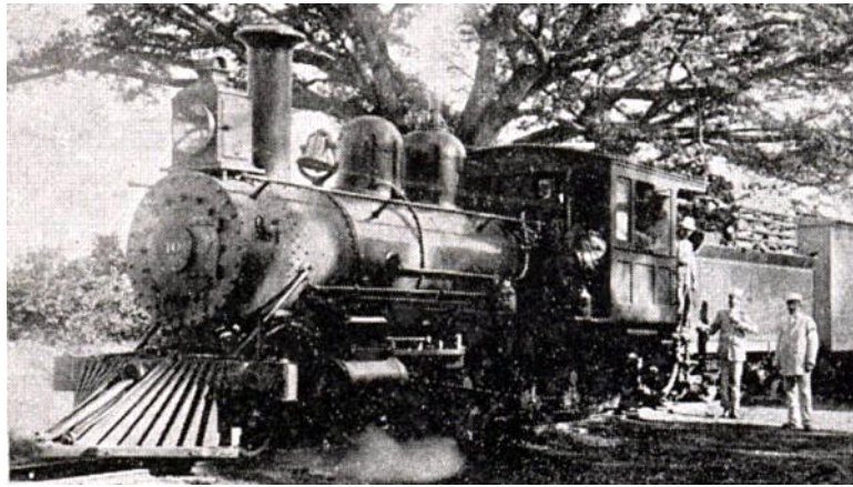
The smokebox number plate carries the number '10'. However, when compared with the works' photo above, this engine seems to have lost its rear sand-dome, and to have gained panelled wooden cabsides.
