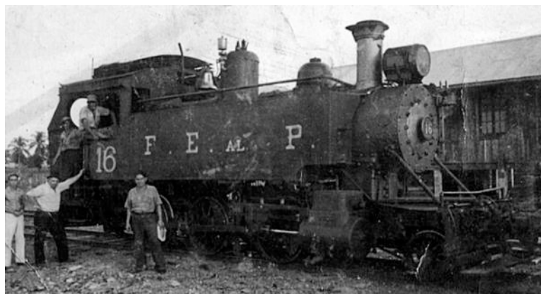
This 2-6-0T numbered 16 might just possibly be a rebuild of the 0-6-OST no. 16 listed above. Certainly the bunker looks similar, and the dome appears rather home-made, as indeed it would have been had the earlier saddle
