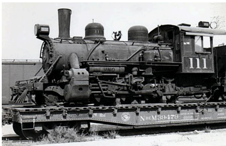
No. 111 aboard a Nacionales de Mexico flatcar whilst on its way to preservation in the USA. Note the bolt-on piston valve chests later fitted to these engines.
