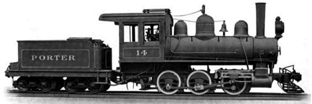
Illustration No. 14, from photograph of 10 x 14 cylinders, coal-burning locomotive, 36 inches gauge of track, exported to Central America for banana plantation.
