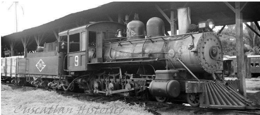
One of the same batch sixty-five years later, in 1961. The changes seem few – a shorter chimney without a cap, the bell moved back close behind the dome, and the oil tank on the tender.
