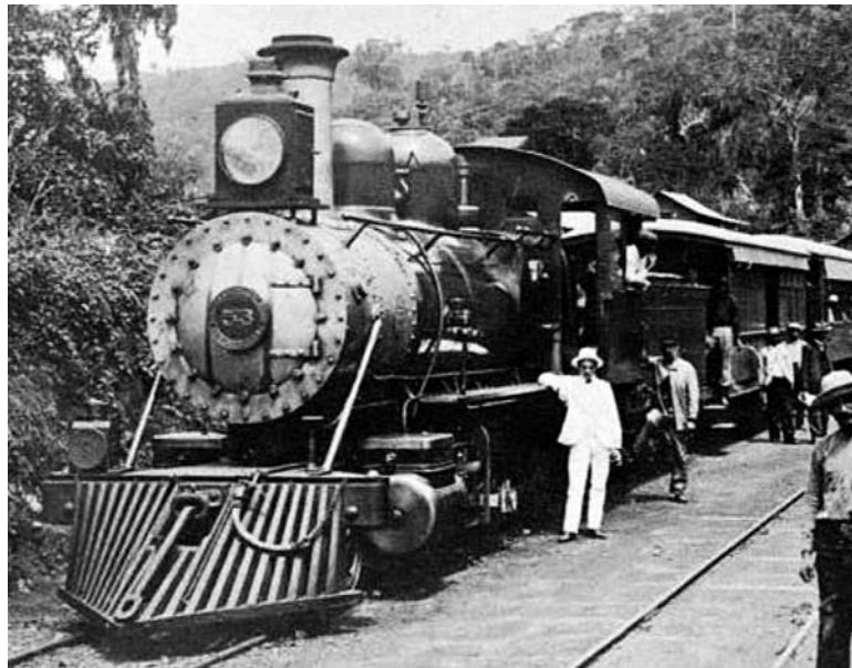
Note the belpaire fireboxes fitted to some of these engines.
