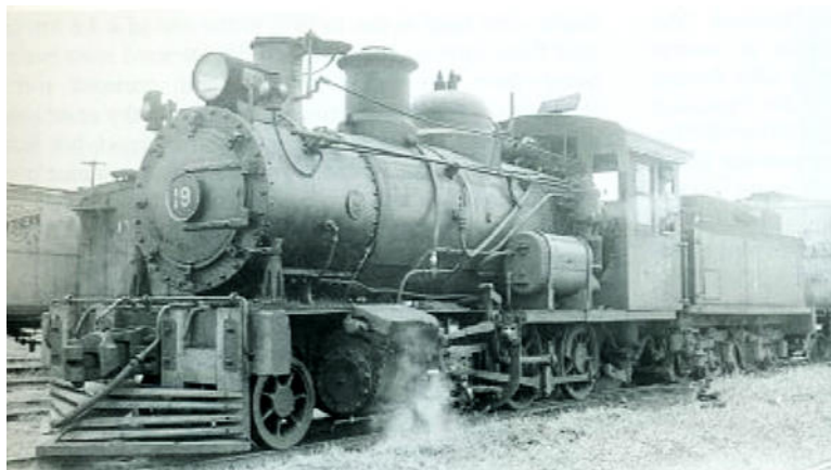
Both of these photos show no. 19 as an example of the Beyer Peacock 2-6-0s rebuilt in the 1920s with replacement Baldwin boilers.
