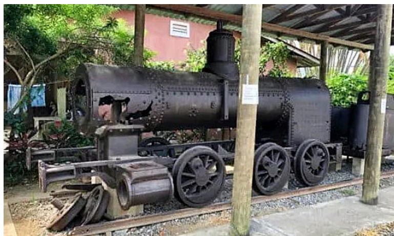
If these remains are from a 3' 6" gauge machine, which is not yet certain, then they probably come from one of the Davenport moguls. The location is at the museum in Omoa. Like the loco pictured above, this one has eleven-spoked wheels, though interestingly without the extra large balance weights on the middle driving wheels that were shown in the previous photo.
