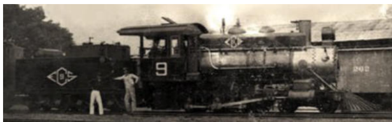
This is a very poor image but it does show 4-6-0 no. 9 with a strange long housing along the top of the boiler on the driver's side. The purpose of this is currently unknown.
