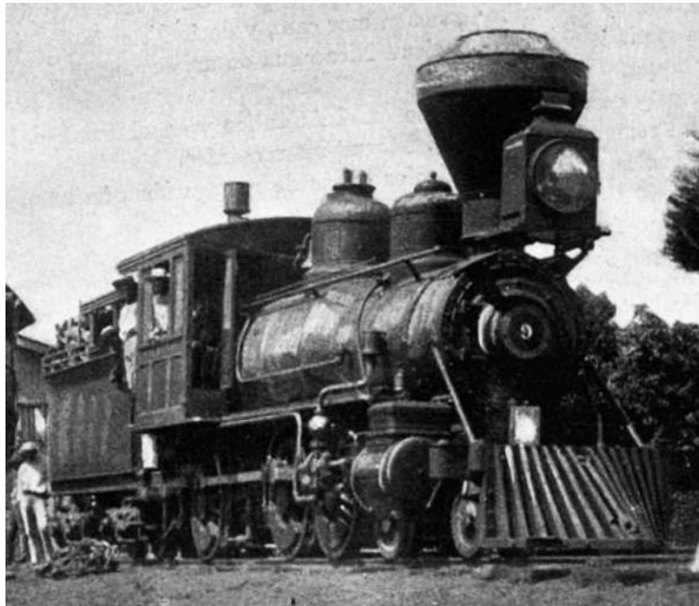
No. 9 seemingly as built with Radley & Hunter spark-arresting stack.
