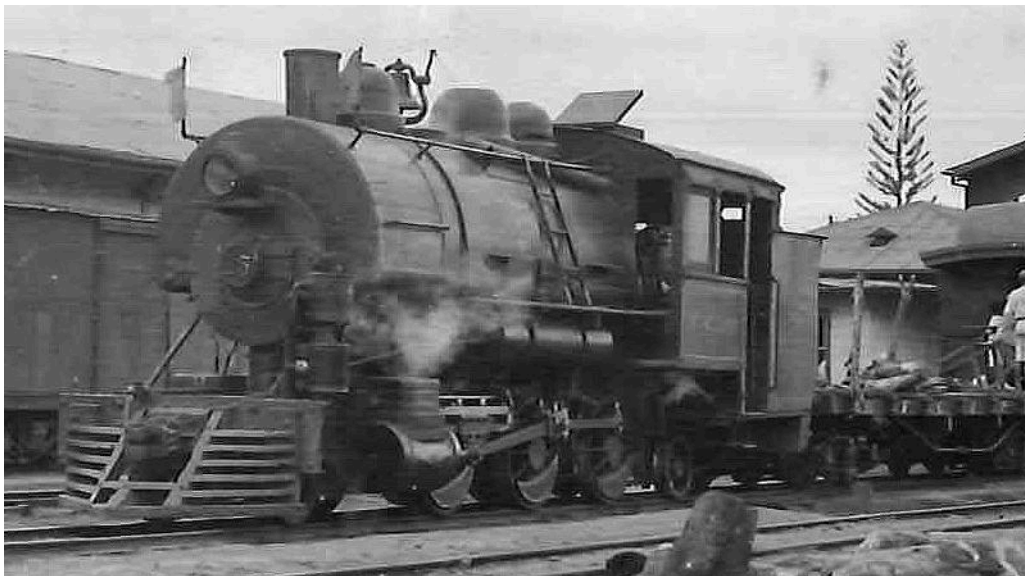
No. 15 seems to have been rebuilt as a 2-6-2ST, using the original saddle tank with a forward extension. Here is the loco in charge of a tourist train from Puntarenas to San José.
