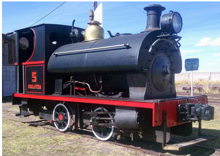
Loco as currently preserved in the museum based in the old loco shed at Guaqui. Note that much of the motion is missing.
