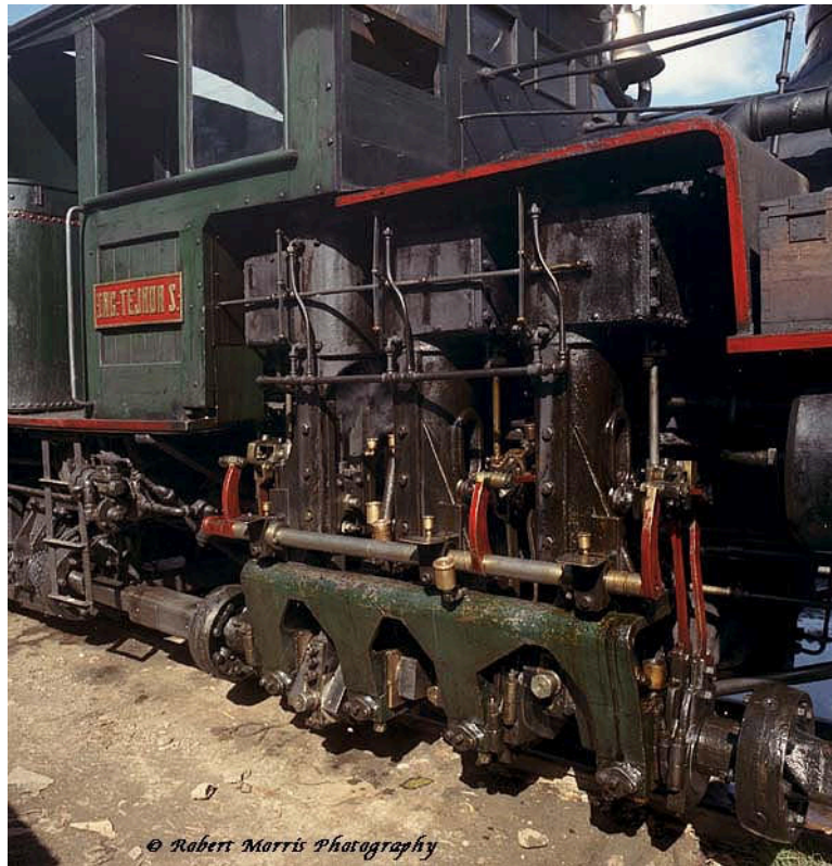
The three cylinder engine of Shay no. 1. Photo by Robert Morris found on the web.
