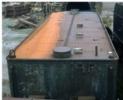
Tenders from the BP Meyers in the works yard at Uyuni in 2000. It will be noted that these were purely water carriers with no built in bunkers, and therefore when these locos were first introduced the extra coal had to be carried in bags on the top – up to four tons of it according to the diagram sheet.
