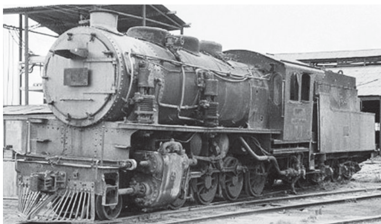
One of the FCALP Borsig 2-8-0s but without the original conical smokebox door with which they seem to have been supplied.
