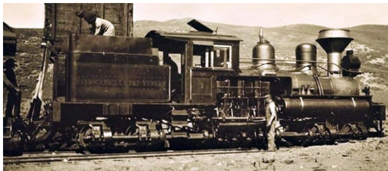
No. 1 is seen here in 1920 near the summit of the line. The tank bears the lettering 'FERROCARRIL LA PAZ-YUNGAS'. Note the Radley & Hunter style stack originally fitted when the locos were wood-burners.
