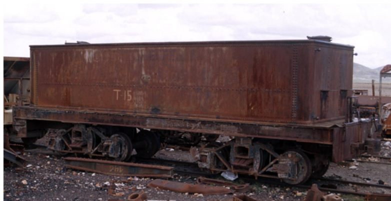
Tenders from the BP Meyers in the works yard at Uyuni in 2000. It will be noted that these were purely water carriers with no built in bunkers, and therefore when these locos were first introduced the extra coal had to be carried in bags on the top – up to four tons of it according to the diagram sheet.
