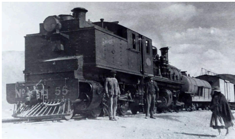
One of the Meyers running with an improvised tender made up of a cylindrical tank mounted on a bogie flat.
